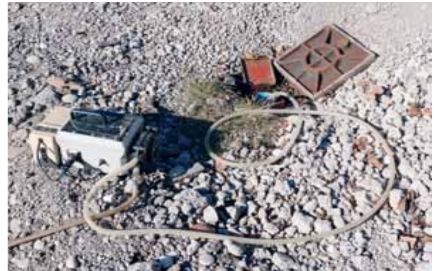
Piezometer inserted in gravel
